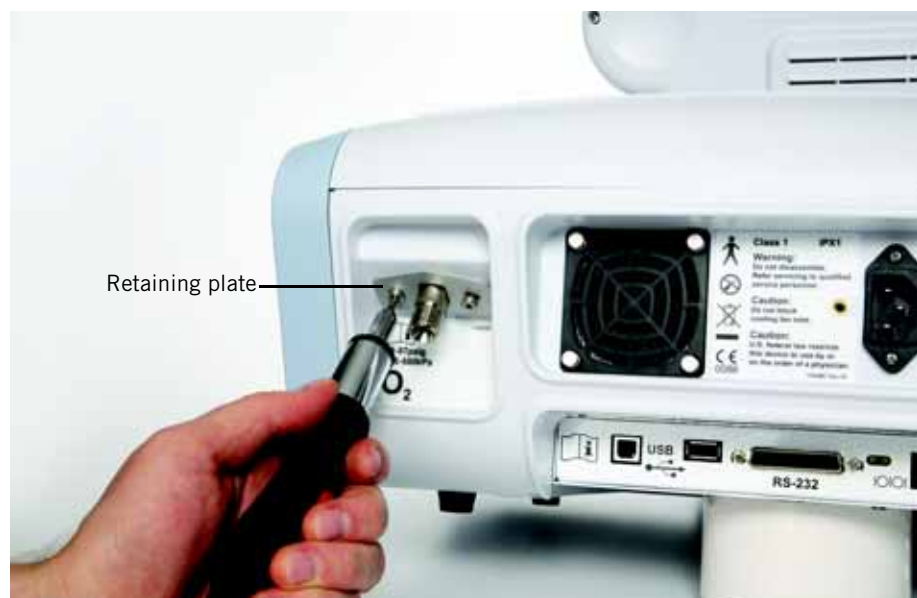
Figure A-3: Installing the oxygen inlet connector
