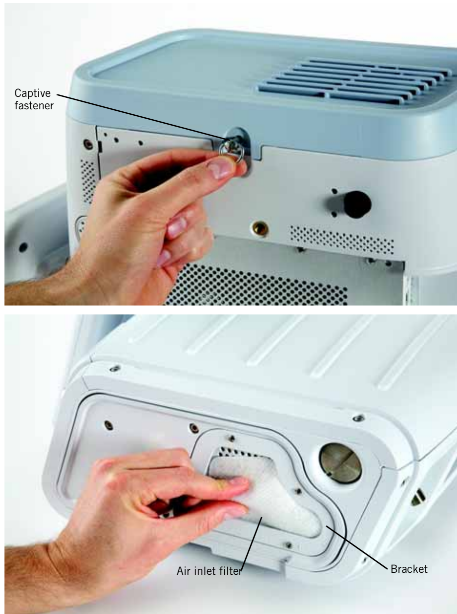
Figure 9-1: Replacing the air inlet filter
